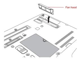
Figure G-2 Removing the Fan hood
